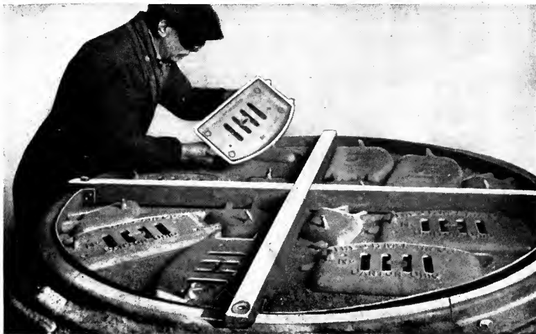
To help some shop officials keep in mind the fact that the cost of a suggested improvement may outweigh its value, one railroad has placed in every shop office signs bearing in large letters the single word, "Cost." Such a policy often leads to the development of devices like that shown below, in which gravity furnishes the required pressure for furnace doors being ground simultaneously
